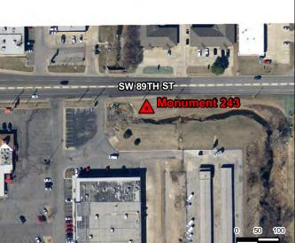
NE Corner of headwall 39.3' NW Power pole 17.8' NW Power pole 66.8' NE Monument 243
