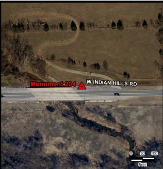
Concrete corner of bridge 47.4' W Power pole 45.3' NE Edge of road 11.5' S
