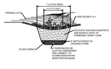
BIOSWALE DETAIL (VEGETATED DRY SWALE)
